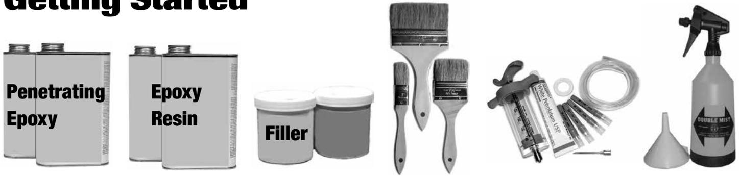
In most cases **Penetrating Epoxy** can be applied with a cheap and **disposable natural bristle brush**. (Do not use foam brushes). Penetrating Epoxy can be mixed in polyethylene and polypropylene containers (plastic paint buckets, margarine tubs, cottage cheese tubs, etc.), and metal containers. Do not use paper containers (cardboard paint buckets), polystyrene (foam) containers, or any disposable drink containers.
