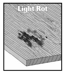
Brush or dab **Penetrating Epoxy** on surface of rot, allowing bad area to absorb all the liquid it can.
