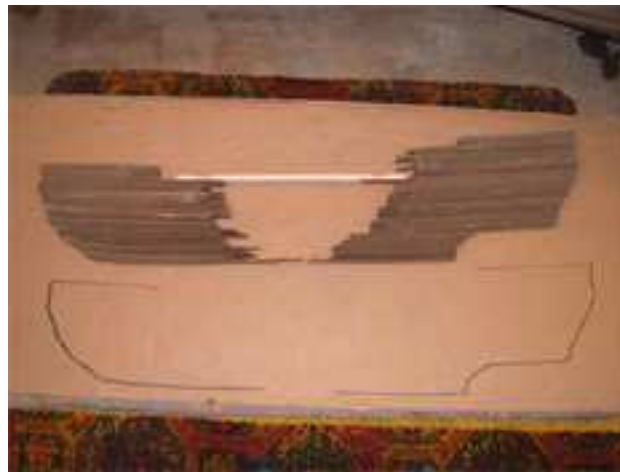
Traced outline was used to fit the plywood strips
